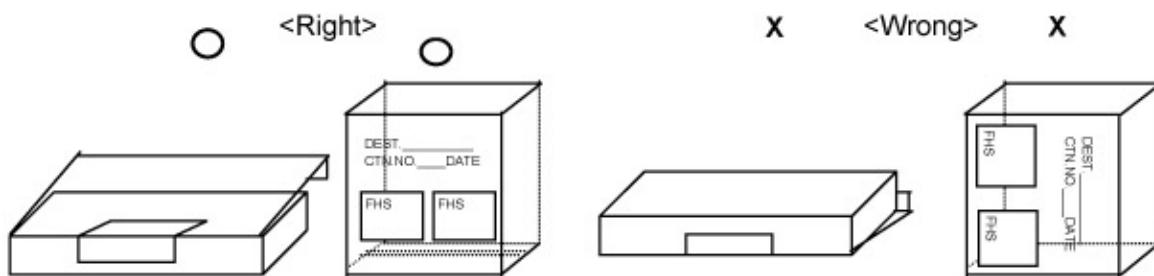
11.3 The inner cartons shall be packed in a cardboard box for transportation.
