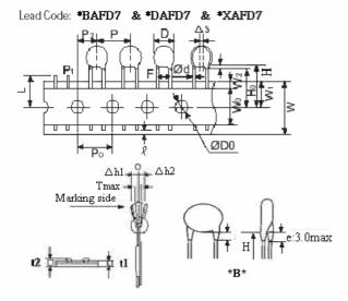
25.4mm pitch/lead spacing 10.0mm taping
