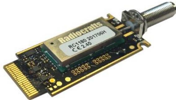
The boards contain an RF module giving wireless connectivity, and the interface circuitry to the host processor in the gateway. The card has an SMA connector for connecting the external antenna.
