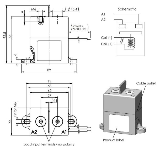
In case of no tolerance shown in dimensional drawing, general tolerances apply: dimension  $\leq 10 \, \text{mm}$ :  $\pm 0.3 \, \text{mm}$ ; dimension  $10 \, \text{to} \, 50 \, \text{mm}$ :  $\pm 0.6 \, \text{mm}$ ; dimension  $> 50 \, \text{mm}$ :  $\pm 1 \, \text{mm}$
